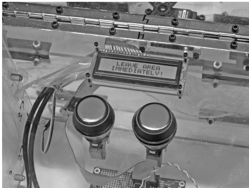
Figure 11-23 The room board LCD display when unsafe air conditions are detected.
