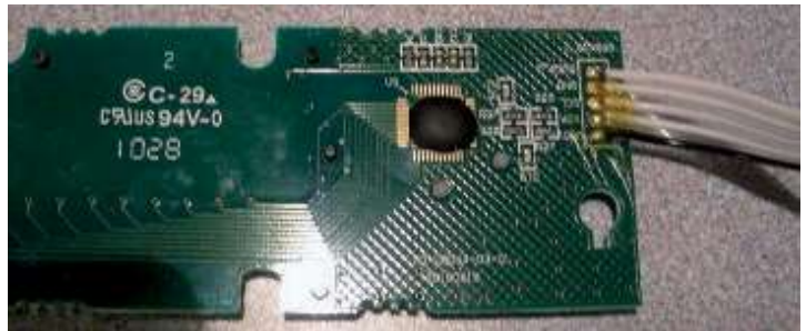
■ FIGURE 3. Neck PCB. To start the MIDI sustain switch function and move the pitch bend/modulation selection switch, desolder and remove the top wire in the ribbon cable. It's labeled "over_d" on the PCB. Next, solder a wire on the underside of the "gnd" wire solder connection next to the "overdrive" hole.
