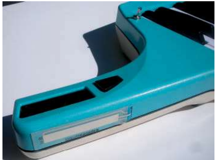
■ FIGURE 6. Softpot mounted on the keyboard neck. Note the hacksaw cut made to accommodate the softpot's flat ribbon cable terminals.
