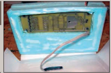
FIGURE C. The Das BlinkenBoard mounted in the foam enclosure.
