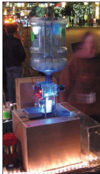
■ FIGURE 5. The Ping Pong Printer with plastic water jug hopper.
