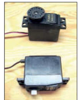
■ FIGURE 5. The position servo with small round horn attached.
