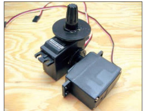
■ FIGURE 8. Winch servo with wire nut glued to the center of the large round horn.
