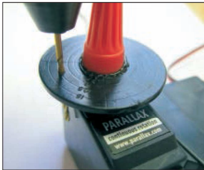
■ FIGURE 9. Drilling a hole where the string to the prop can be attached.
