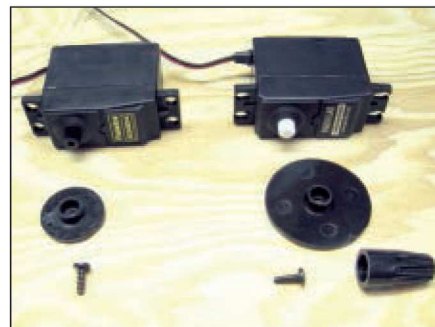
■ FIGURE 4. The position servo (left) and the winch servo (right) ready for assembly.
