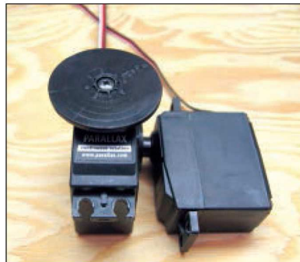
■ FIGURE 7. Winch servo with the large round servo horn in place.
