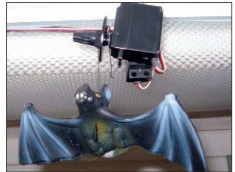
■ FIGURE 11. The Prop Dropper in place with a prop wound up and ready to drop.
