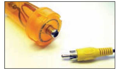
■ FIGURE 21. Female RCA jack mounted on the pill bottle cap ready for connection.
