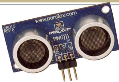
■ FIGURE 1. PING)))™ Sensor. The Parallax PING))) sensor uses ultrasonic soundwaves to determine the distance to an object and returns a value in milliseconds that is quite accurate. It only requires three connections: 5V+, GND, and a single TTL level pin for both sending and receiving data.
