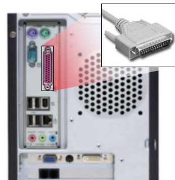
Illustration 1: a “DB25” Parallel Port
