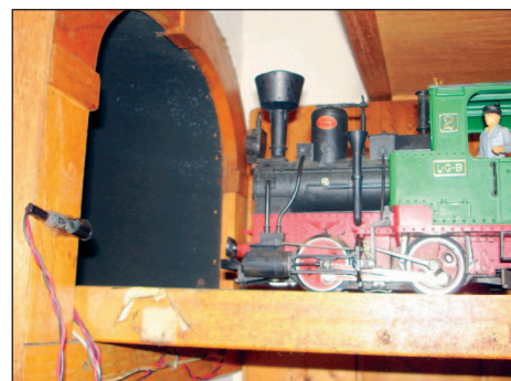
■ FIGURE 13. The IR beam-break sensors mounted on the train tunnel entrance.
