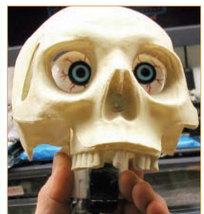
■ FIGURE 8. Front view of skull with servo operated eyes.
