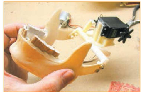
■ FIGURE 5. The new servo motor in place in the jaw.
