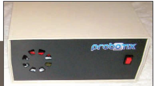
■ FIGURE 6. The Ready To Run case contains the power supply and the motor controllers.
