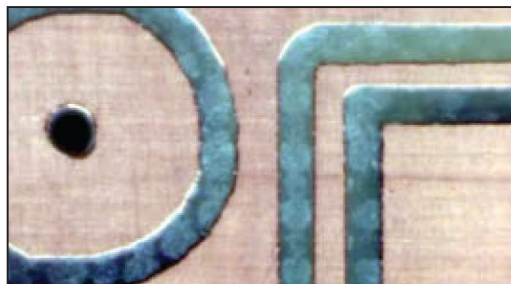
■ FIGURE 17. Test cut #2 shows the Z axis at the correct depth. Note the underlying PCB board material is mostly intact.
