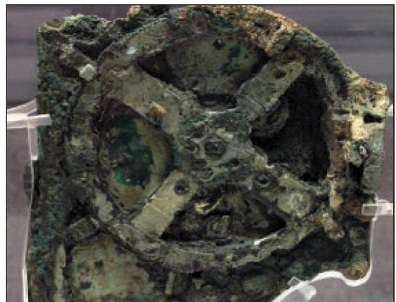
■ The Antikythera mechanism is an ancient mechanical device designed to calculate astronomical positions. Scientific examinations place its date of creation to be between 150–100 BC.
