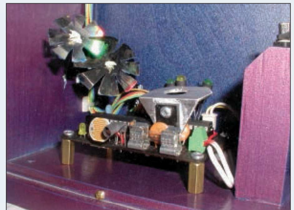
■ The PCB hosts LEDs, CDS cells, IR Emitter/Detector pair, and prismatic flowers.
