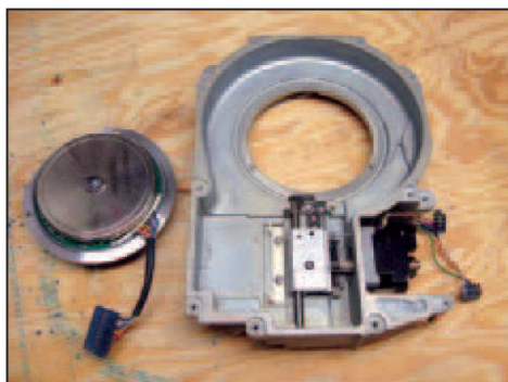
■ FIGURE 3. This is what's left after removing the platters, platter drive motor and circuit board from a dead ST-506 hard drive.
