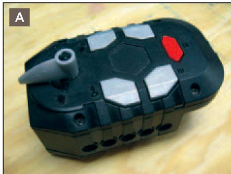
■ FIGURES 2A, 2B, and 2C. The LEGO Spybotics remote control module sports a nice AAA battery box, IR transmitter, pushbuttons, and an LED.
