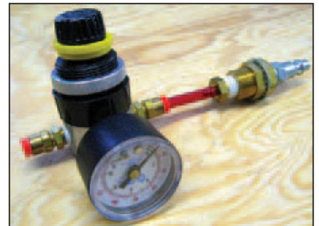
■ Figure 21. All the parts to connect the 1/4 inch "NTP" style workbench compressor to the robot arm.
