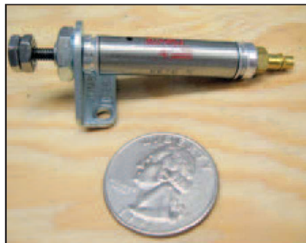
■ Figure 9. A dual-acting guided cylinder with 1" of travel.
