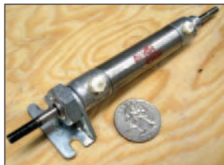
■ Figure 9. A dual-acting guided cylinder with 1" of travel.
