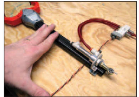
■ Figure 20. The finished pneumatic gripper with solenoid valve connected. Those with sharp eyes may notice that I swapped the 90 degree barb-connectors for straight-through connectors so the assembly would lie flat for the photo!
