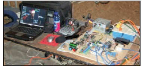
■ The upgraded "PONGINATOR MK3" control system incorporating ideas from MK1 and 2.
