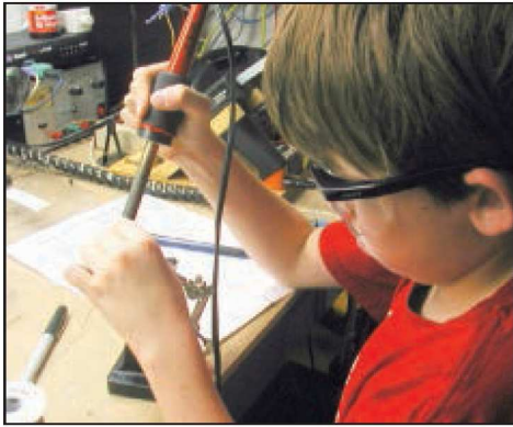
■ Nic Graner learning to solder at age nine. One of the first things he was taught was to always wear safety glasses!
