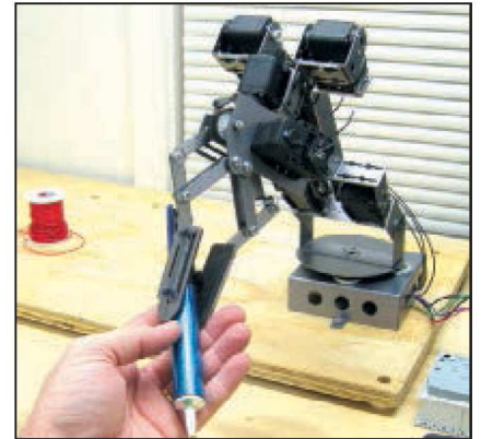
■ FIGURE 13. A slight tug removes the solder vac from the AX-12+ gripper.
