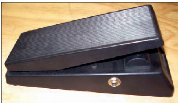
■ FIGURE 14. Foot pedal control expected to add hands-free control to the AX-12+ motions.
