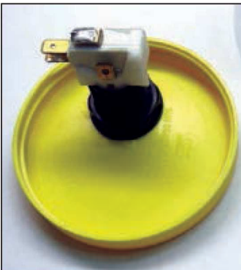
■ FIGURE 8. Lighted push-button mounted in jar lid.
