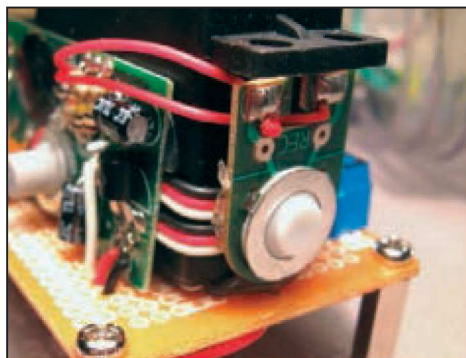
■ FIGURE 18. The record button hot-glued to side of servo.
