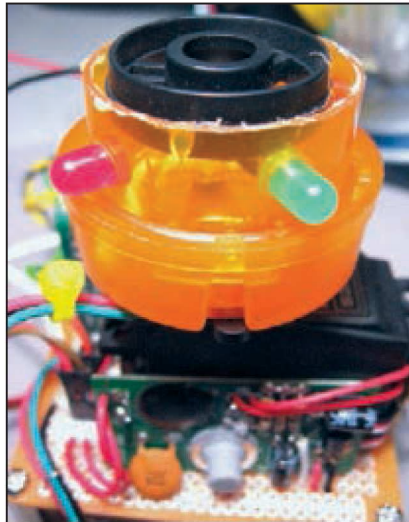
■ FIGURE 21. Tire hub from an old toy glued to the top completes the scan head.
