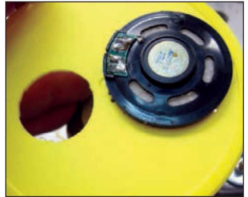
■ FIGURE 12. Speaker hot-glued to the bottom side of the jar lid.
