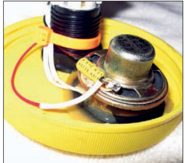
■ FIGURE 22. Second speaker piggy-backed on top of first speaker creating a "mechanical mixer."
