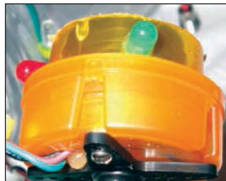
■ FIGURE 19. Scan head with LEDs mounted and servo horn attached.
