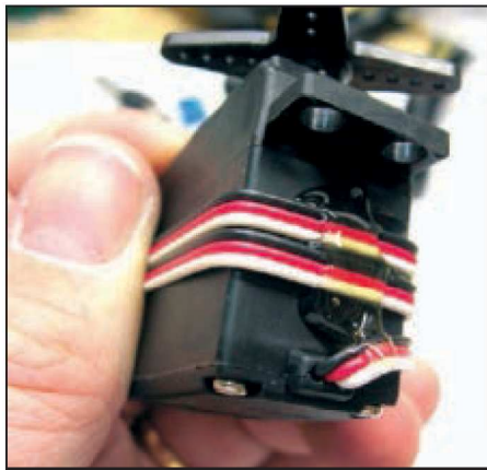
■ FIGURE 3. Excess wire wrapped around the servo and hot-glued in place.
