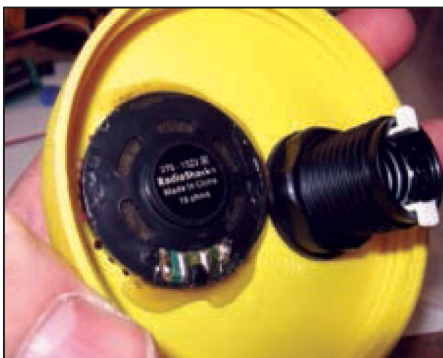
■ FIGURE 13. Pushbutton test-fit next to speaker.
