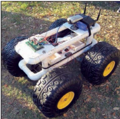
■ PHOTO 10. Bob Comers robot made from PVC pipe and recycled "kiddie car" motors and wheels.
