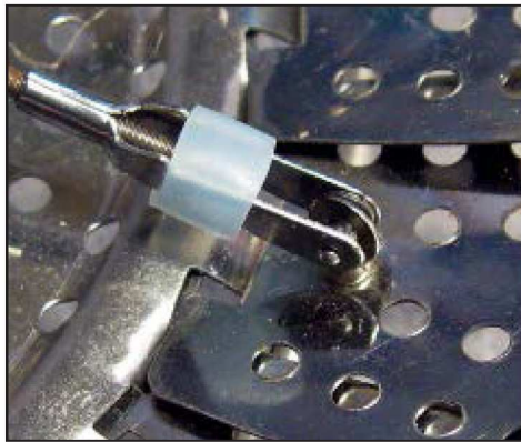
■ FIGURE 11. Solder one of the washers (included in the ball links package) into the slot of a small machine screw.
