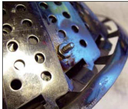
■ FIGURE 12. Insert the washer/screw combo into one of the holes on a petal (as shown) and tighten a nut on the outside of the petal.
