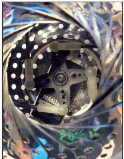
■ FIGURE 16. The Power Flower should be able to fully open and close after adjusting the petals and hinges where the petals meet the base.
