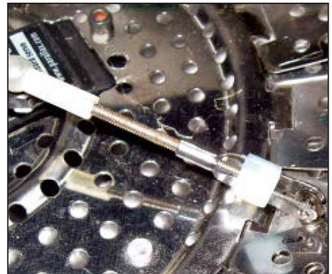
■ FIGURE 13. Attach the clevis to the washer/screw combo to anchor the rod to the petal.
