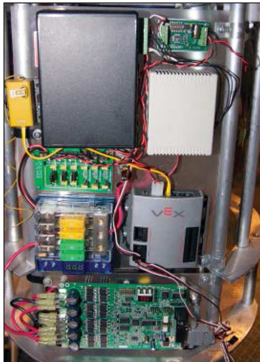
■ FIGURE 6. Chris James' R2-D2 internal wiring and control electronics.
