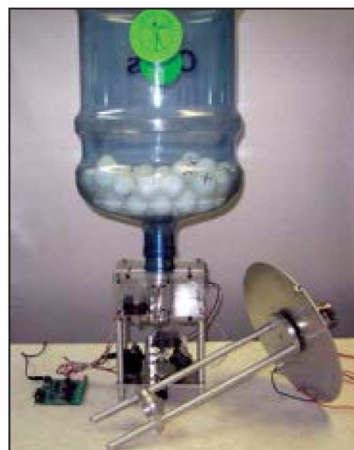
■ FIGURE 6. PingPongPrinter prototype (shown here with agitator removed and placed in the foreground for clarity).
