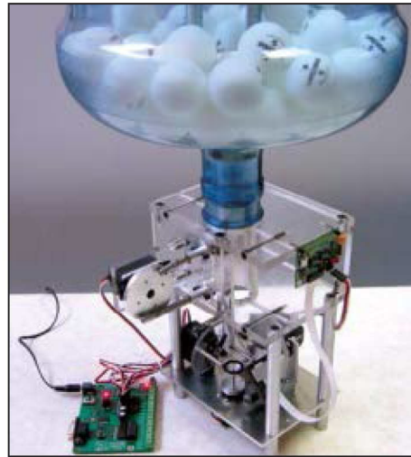
■ FIGURE 12. PingPongPrinter loaded and ready to print.
