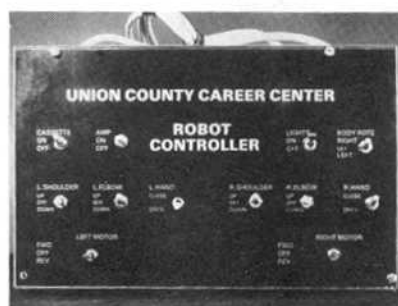
FIG. 38—COMMAND CONSOLE provides the means for controlling remotely via cable.
