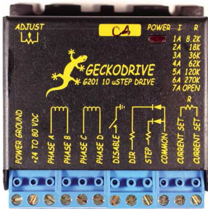
PHOTO 2. Here's a look at the G201 as it would appear out of the box. The screw terminals are removable to aid in mounting the G201 to an external heatsink.
