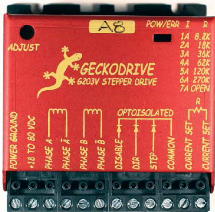
PHOTO 4. The G203V Vampire is pin-compatible with the G201 with the exception of the COMMON terminal, which is referenced to the controller's ground on the Vampire. Note also that the PHASE names are more stepper motor datasheet correct than the G201's PHASE A, PHASE B, PHASE C, and HASE D nomenclature.
