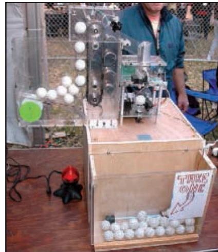
■ PHOTO 12. The Ping Pong Printer with its new ball-feed hopper by Rick Abbot.
